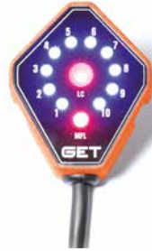
LAUNCH AND TRACTION CONTROL SYSTEM
